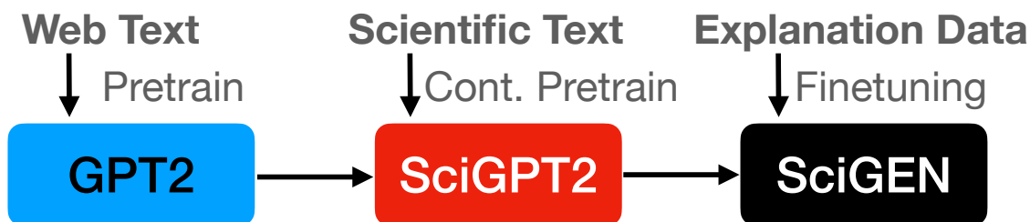
Figure 2.2: Overview of the construction of SCIGEN. We take the pretrained GPT2 and continue pretraining on scientific texts. We then finetune using data in Table 2.1.
